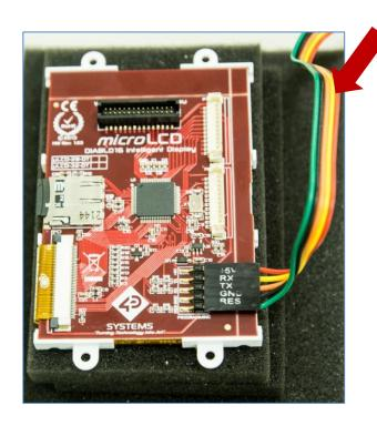
5-way cable connected to the µUSB-PA5
