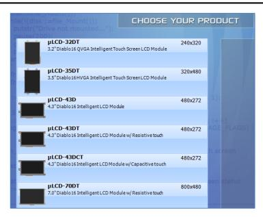
Select the appropriate screen and preferred orientation. The screen used in this example is a **uLCD-32DT** (landscape reversed orientation).
