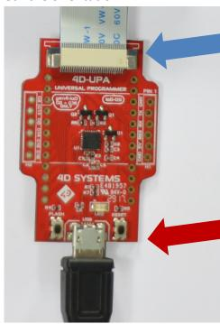
FFC Cable Connected to the 4D-UPA (Silver side facing upward)
