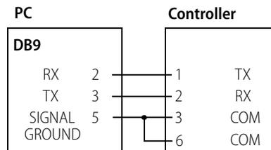
\* Minimum requirements for wiring an RS-232 serial cable to connect to a PC. If you want to connect the controller to a modem, see form #1595, the *SNAP PAC R-Series Controllers User's Guide*, for all eight pin connections.
