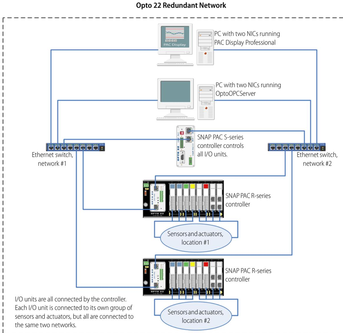
This diagram shows two SNAP PAC R-Series controllers functioning as I/O unit brains connected to two separate Ethernet networks. This configuration addresses the concern that an Ethernet network may fail or need maintenance, leaving the PC running OptoOPCServer and OptoDataLink, the PC running PAC Display, the controller, and the I/O units unable to communicate.
